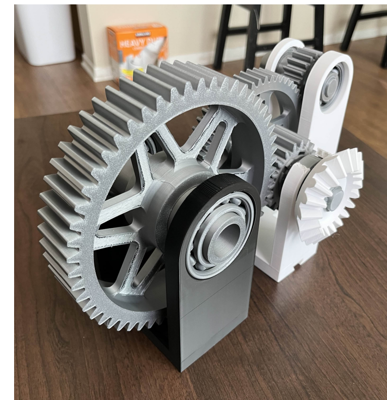
Gear Layout and 3D Printed Proof of Concept
