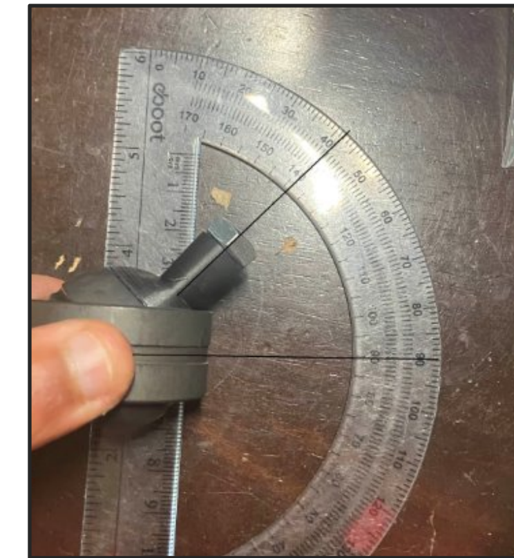
Fig 3: Custom Misalignment Spacer (42°)
